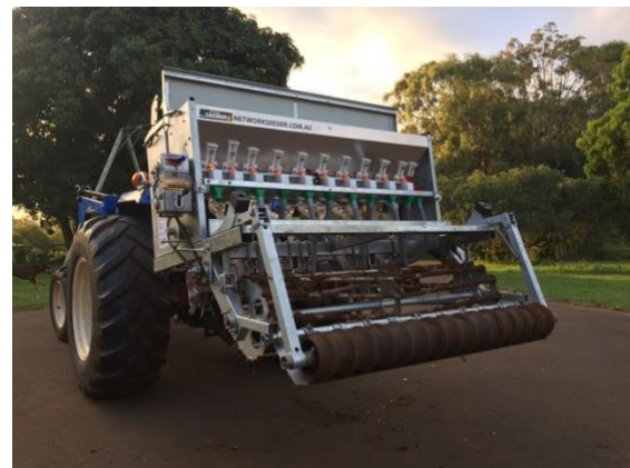
Photo 3: The Network Seeder is 1.4m wide. For this trial the centre strips were seeded at 1.2m.
